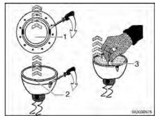
Fig. 203 Changing the halogen bulb
