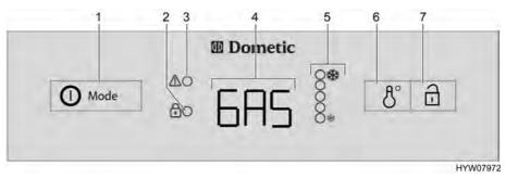
Fig. 159 Operating controls for the refrigerator (Dometic 8 series with AES)
