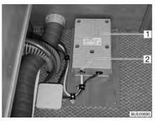
Fig. 137 Transformer for electrical floor warming unit
