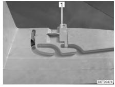
Fig. 67 Ventilation position locking mechanism
