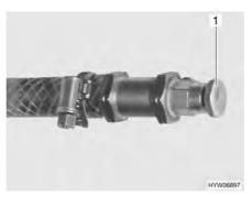
Fig. 197 Bleeding valve of hot-water heater
