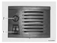
Fig. 139 Operating controls for auxiliary heat exchanger
