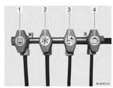
Fig. 127 Symbols for the gas isolator taps
