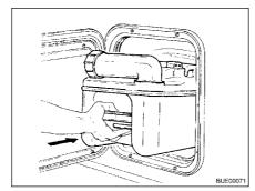
Fig. 190 Inserting the Thetford cassette
