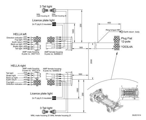
Fig. 126 Circuit diagram, exterior
