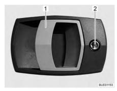
Fig. 26 Door lock of conversion door, outside
