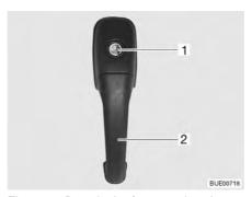
Fig. 24 Door lock of conversion door, outside
