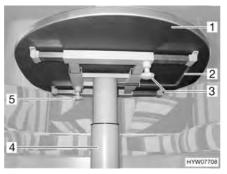
Fig. 77 Lift-off table
