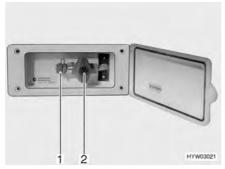
Fig. 96 External gas connection, gas isolator tap closed
