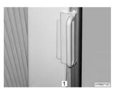
Fig. 21 Locking mechanism for Roman shade on driver's/front passenger's windows
