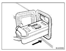
Fig. 179 Inserting the Thetford cassette
