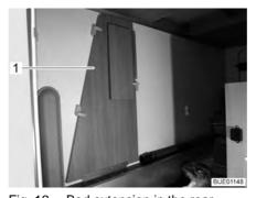
Fig. 12 Bed extension in the rear garage
