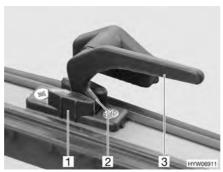
Fig. 56 Catch lever in the "continuous ventilation" position
