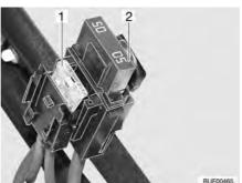
Fig. 112 Fuses on the starter battery
