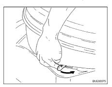
Fig. 183 Operating the sliding trap
