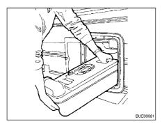
Fig. 176 Removing the Thetford cassette
