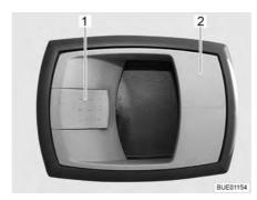
Fig. 27 Door lock of conversion door, inside
