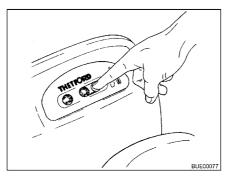
Fig. 186 Closing the sliding trap
