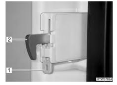
Fig. 163 Lock hook fixture
