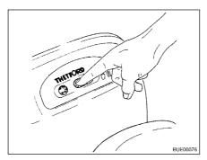
Fig. 185 Opening the sliding trap
