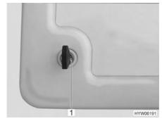
Fig. 32 Push-button lock service flap
