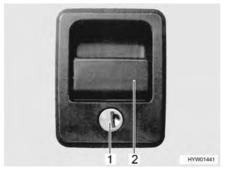
Fig. 30 Flap lock with recessed handle
