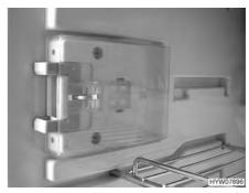
Fig. 165 Locking device in ventilation position
