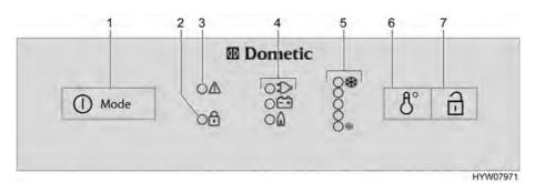
Fig. 158 Operating controls for the refrigerator (Dometic 8 series with MES)
