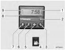
Fig. 140 Operating unit for independent vehicle heater
