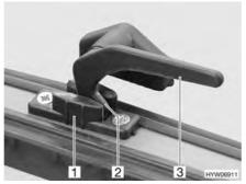
Fig. 71 Catch lever in the "continuous ventilation" position
