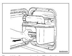
Fig. 187 Removing the Thetford cassette
