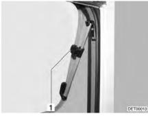
Fig. 70 Skylight with rotary hinges, open
