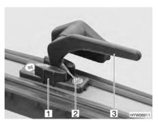
Fig. 59 Catch lever in the "continuous ventilation" position
