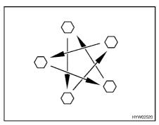
Fig. 210 Tighten the wheel nuts or wheel bolts cross-wise
