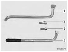
Fig. 211 Wheel bolts with on-board tool set
