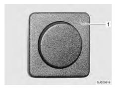
Fig. 47 Recessed halogen light
