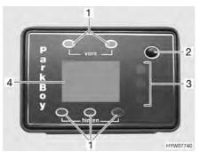
Fig. 15 Parking distance control operating unit
