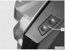
Fig. 162 Release button of the refrigerator door (Dometic 8 series)
