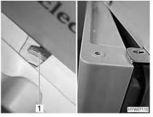
Fig. 161 Refrigerator door/freezer compartment door in ventilation position (Dometic 7 series with separate freezer compartment)
