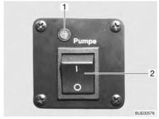
Fig. 136 Operating switch for auxiliary circulating pump
