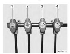
Fig. 95 Symbols for the gas isolator taps
