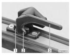
Fig. 54 Catch lever in "closed" position
