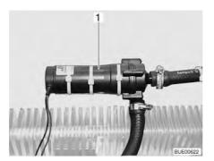
Fig. 135 Auxiliary circulating pump
